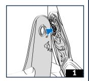
1 – Locate the visor notch system on each of the side plates of the visor mechanism.
